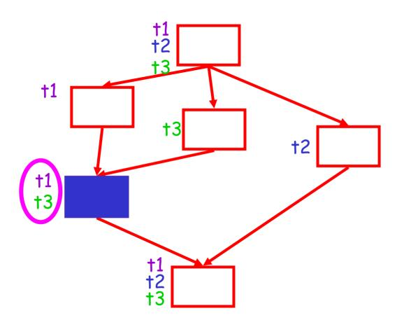
Label each node of the control flow graph with the set of tests that reach it.
